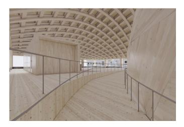
The main roof consists of a Free Form construction that spans a footprint of 25 x 48 metres. The planning, production and execution of the highly complex roof geometry were handled by the Free Form specialists at Blumer Lehmann, together with their partners.
